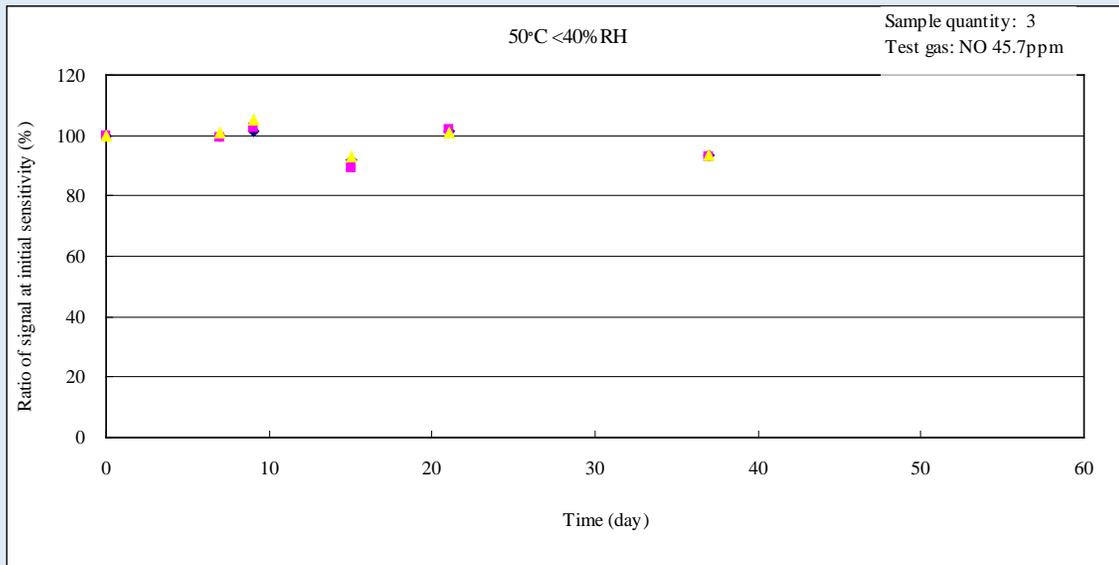
**High Temperature / Normal Humidity:** The following graph illustrates the typical signal output stability for a sensor exposed to +50°C and 60% RH over 50 days. The NO concentration used was 45.7ppm NO in air.
